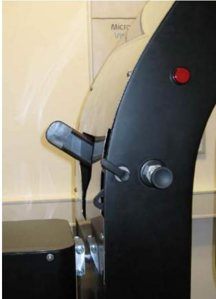
Stop position for horizontal canal DPRM.
