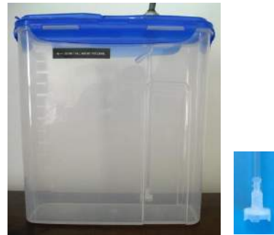
Figure 4 External tank with pick up filter
