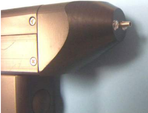
Figure 5 Place silicone tip on irrigation handle nipple. Use silicone Tips provided by Interacoustics that are calibrated for flow rate and heat transfer.
