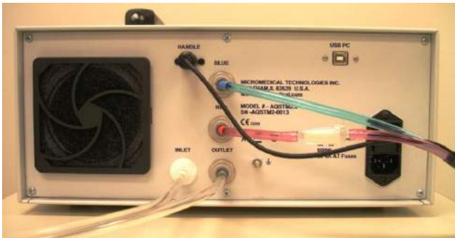
Figure 3 Tubes and Electrical Connection
